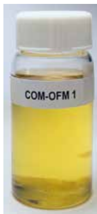
OFM1 > 0.5% shows globule residue at bot- tom of sample vial after 8 hrs mixing both room temp and -20°C
